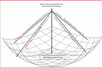
A 4-dimensional plot is used to visualize multiple values (dimensions) relative to one another simultaneously. Each dimension is plotted along its corresponding axis. The magnitude of the system performance is then projected from the apex (origin). Systems that are closer to the apex perform better than those further away.
